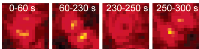
FIGURE 5. Emission patterns taken from a series of consecutive defocused images recorded for a single C1P4p in a 100 nm Zeonex film. Images were recorded at 1\ \mu\text{m} defocusing to the glass surface. Time intervals, during which successive patterns have been observed, are listed underneath the images. The emission pattern of a single C1P4p molecule changes as function of time. The patterns provide direct evidence that different chromophores of the C1P4p emit in time as different dipole orientations.
